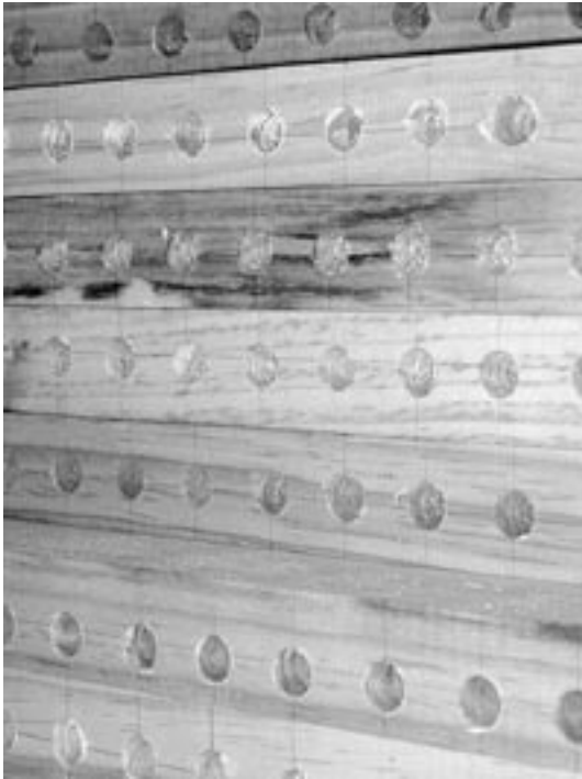
Photo 2. Pinus radiata boards (35 mm thick), drilled and ready for the cores to be glued.
