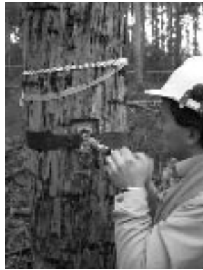
Measurement of growth strain in a standing tree is undertaken by Juan Carlos Valencia of the University of Tasmania (UTas)
