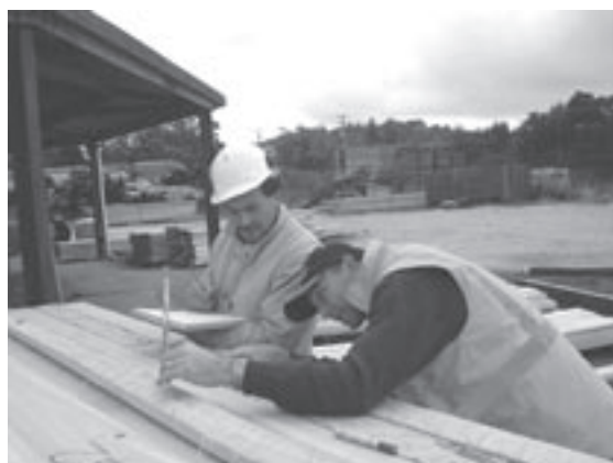
Juan Carlos Valencia (UTas) and Dr Peter Volker (FT) measure boards for distortion after sawing.
