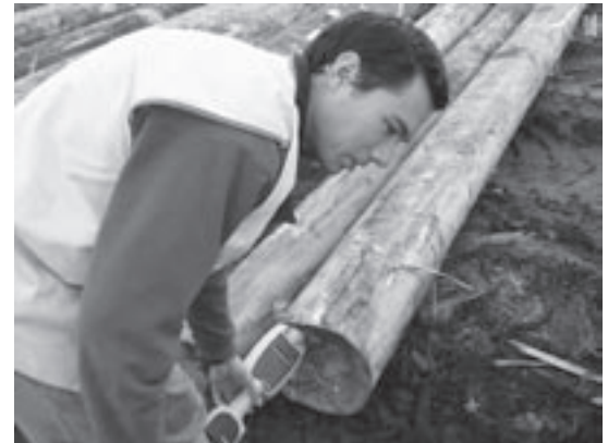
Dr Trevor Innes (UTas) measures acoustic velocity in logs.
