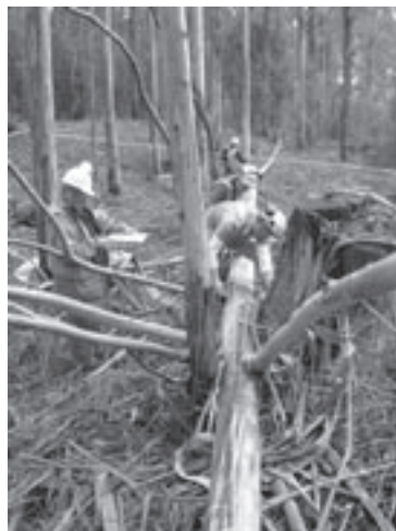
Collection of detailed tree measurements on tree height, upper stem diameters, branch size, location and direction were made after felling.
