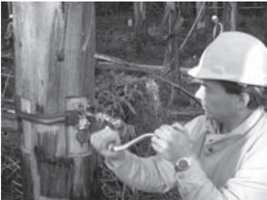
Juan Carlos Valencia (UTas MSc student) collects growth strain measurements from standing trees.
